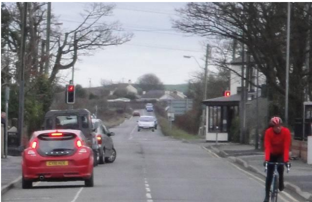
Footbrake on when stopped creates light pollution at high level directly into a driver's eye
