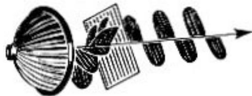
**Figure 6.** Plane polarized light produced by placing a polarizing filter in an ordinary light beam.
