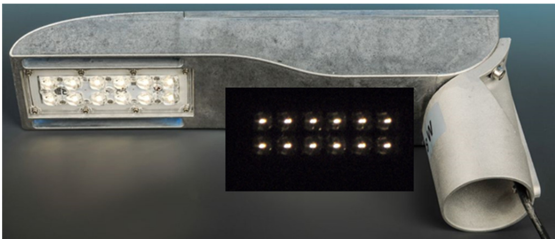
Figure 15: One of the LED street lights tested. The inset shows a light controlled photographic image of the LED chips under attenuation by 6 orders of magnitude. Note that similar hotspots were observed on all the models tested.
