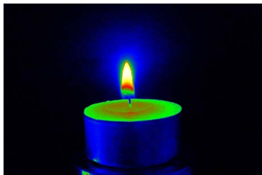
Figure 1 – Substantially uniform illumination from a candle shown in the yellow region of the flame.
